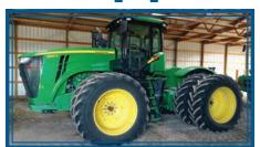
\*2012 John Deere 9360R 4 wheel drive tractor, 24/6 Manuel shift trans., color touch display, Deluxe command view II cab,5 remote cylinder, low flow, 2-165# & 8 450# weights, NO PTO, 620/70R42 tires and duals, 2140 hours, been through JD inspection, very nice tractor
