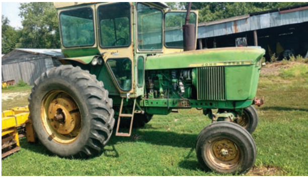
*1970 John Deere 4020 Diesel Tractor WF, cab, dual hyd. 3-pt., 18.4x34 rear rubber, 4 sets rear wheel weights, SN 230153
